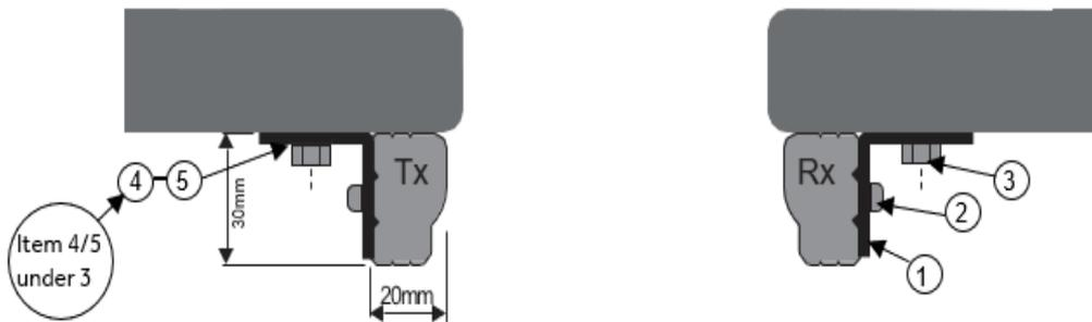
Install the TX and RX edges onto the doors using the mounting brackets on each edge spaced at regular intervals or as convenient if existing hole positions exist.
