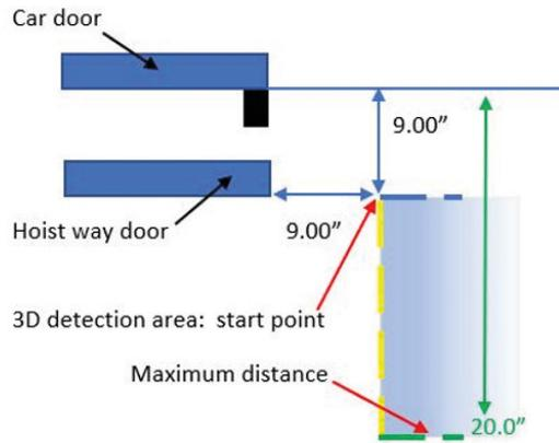
Only shown in the diagram to the right for the TX unit, (Left side of elevator) but same distance criteria is applied to RX unit. (Right side of elevator)
