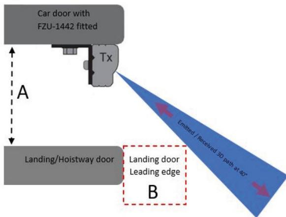
The landing door leading edge, point B can be calculated from the car to landing door distance, point A and the 3D emitted/received angle of 40°.
