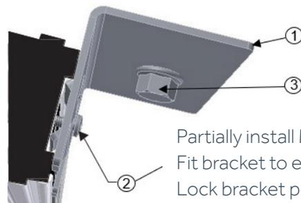
Partially install M3 x 6mm thread forming screw to bracket.
