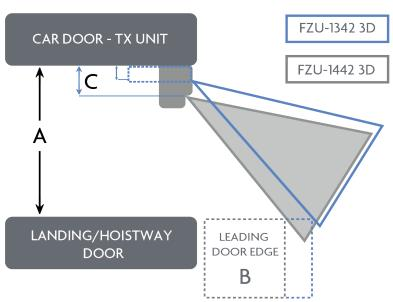
If a more detailed distance needs to be calculated then door leading edge B can be calculated using the following formula:
