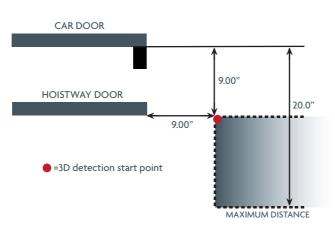
The diagram shows the TX unit only (left side of elevator) but the same distance criteria is applied to the RX unit (right side of elevator).
