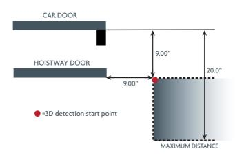
The diagram shows the TX unit only (left side of elevator) but the same distance criteria is applied to the RX unit (right side of elevator).
