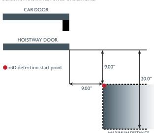
The diagram shows the TX unit only (left side of elevator) but the same distance criteria is applied to the RX unit (right side of elevator).
